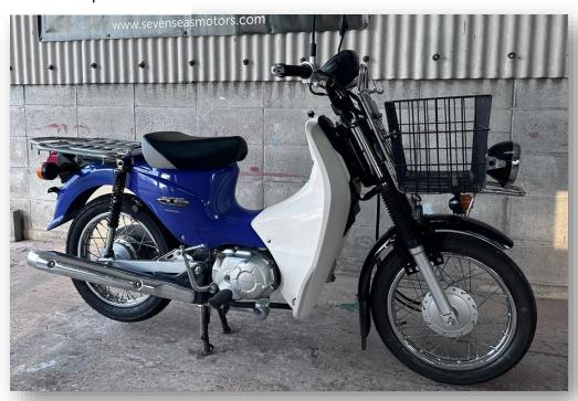
The C110 is basically a modernish version of the C90 but with a larger engine, fuel injection and telescopic front forks.
